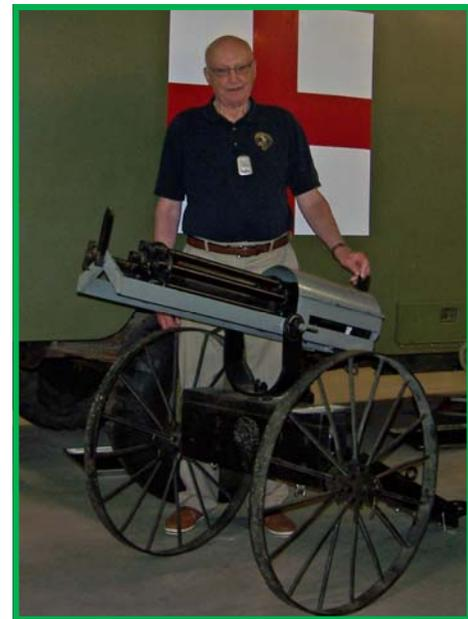
The Gatling gun. It had several barrels, fired in succession, turned by a hand crank. On the modern version called a mini-gun, used on helicopter gun ships, the barrels are turned by an electric motor.
